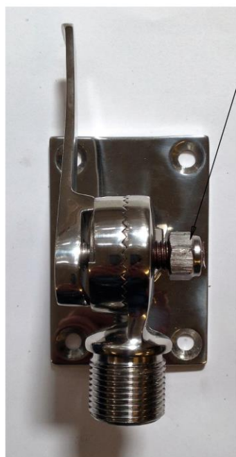
1: Loosen Lock nut
