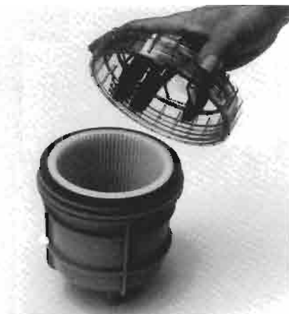
Controle koelwaterfilter. Checking the raw water strainer.
