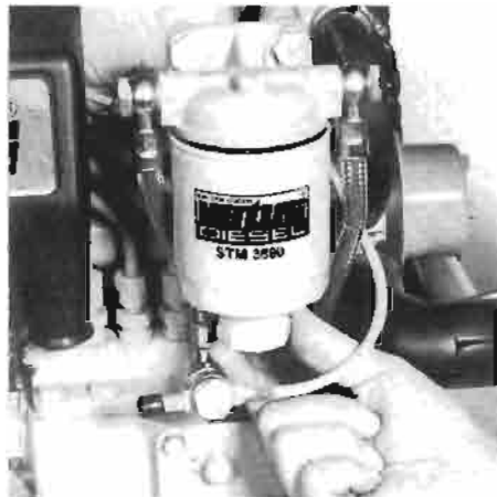
Waterafscheider aftappen. Draining water separator.
