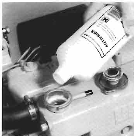
Vullen koelsysteem. Filling of cooling system.
